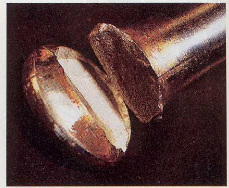
Crevice corrosion in stainless is often found in areas hidden from view. Some examples: a rudder pin that looks as if it was attacked by teredo worms ( below, left ), a keelbolt from a wooden boat ( above, left ), and a rod-rigging cold bead from a large yacht ( right ). In all cases, the corrosion could only be observed by disassembly.
